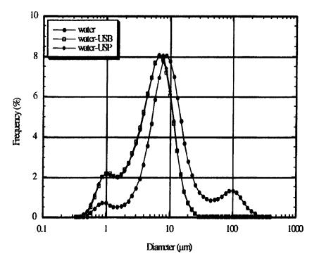
Comparison of the particle size distribution of UF-TATB samples suspended in deionized water with samples suspended in deionized water plus the use of an additional powder dispersion method.
