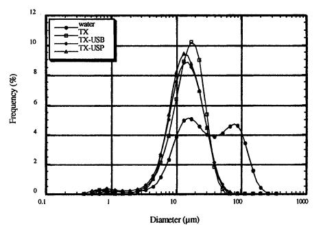
Comparison of the particle size distribution of FP-TATB samples suspended in deionized water with samples suspended in deionized water plus the use of an additional powder dispersion method.
